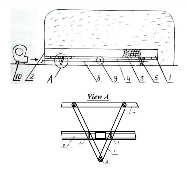
Fig.1 Scheme of installation for drying stem agricultural products
