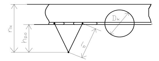
Fig.2 Calculation scheme for determining the height of the control support and the diameter of the installation wheel
