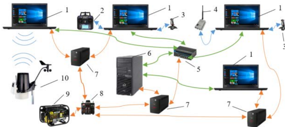
Fig 7. Interconnection of operator workplace equipment
