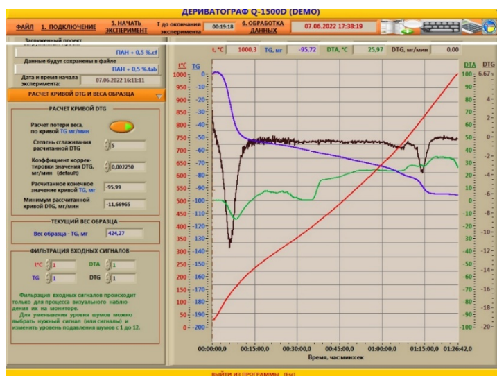
Fig. 4. DTG of 15% aqueous dispersions of montmorillonite clays of the Darbaza deposit in the presence of 0.5 % synthesized sulfonic acid WSP
